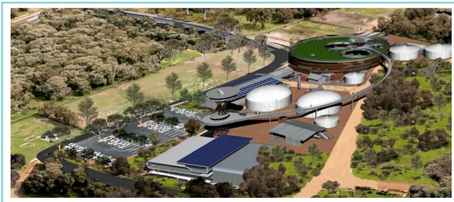
Figure 1: 3D model showing the integrated bio-resource recovery facility. Modular integrated wastewater, biogas and biofertiliser plants.
