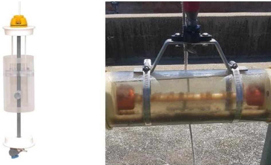
Figure 1: Kemmerer (left, vertical arrangement) and Van Doorn (right, horizontal arrangement) sampler
